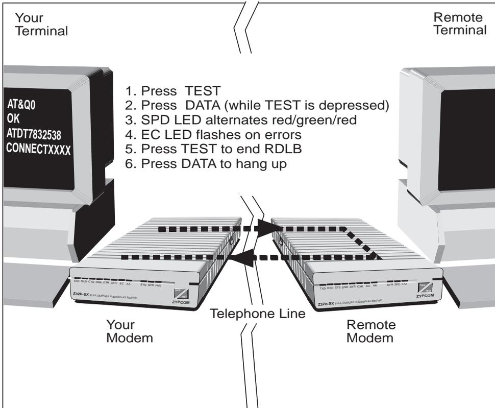
**Figure 10-5. Remote Digital Loopback Self-Test**
