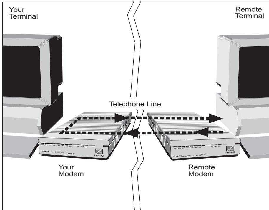
**Figure 10-3. Local Digital Loopback Data Test**
