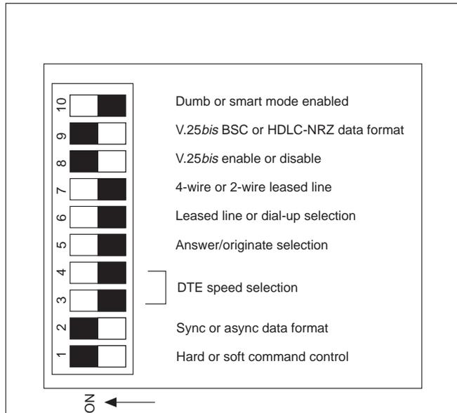
Figure 7-1. Using the DIP Switches to Select V.25bis
