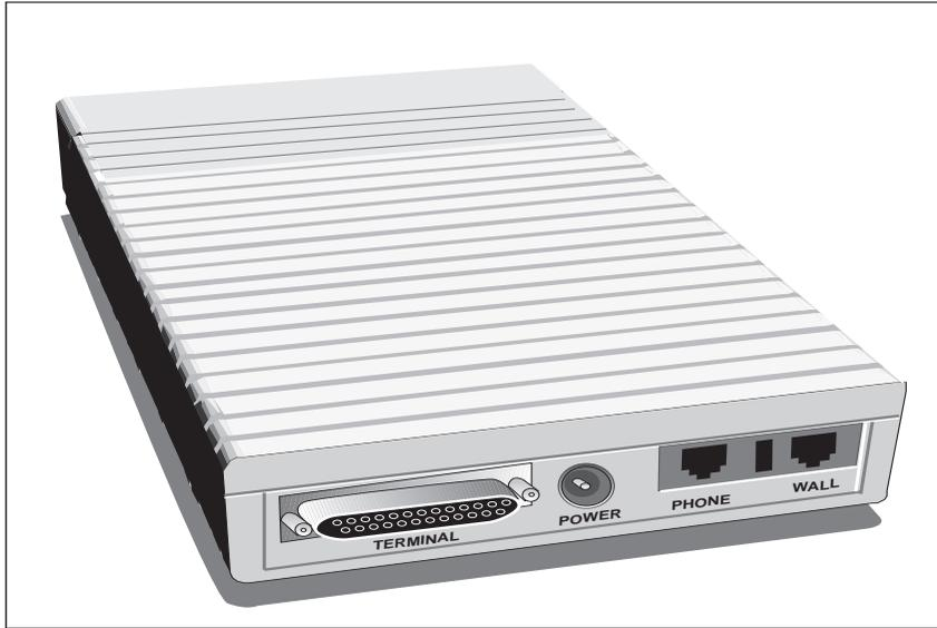
*Figure 1-2. SX-Series and SE-Series Rear Panel*
