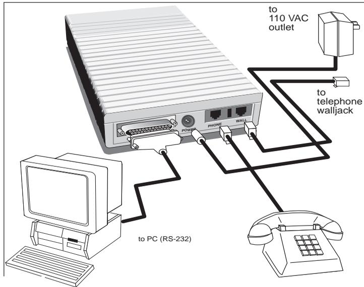
**Figure 3-1. Dial-up Modem Connections**
