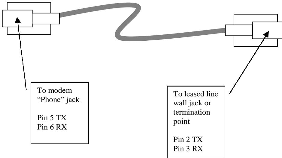
**Figure 8-4. SX-Series or SE-Series 2-wire Leased Line Cable**
