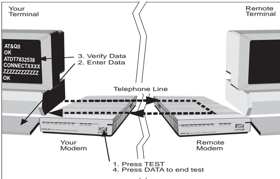
Figure 10-4. Remote Digital Loopback Data Test
