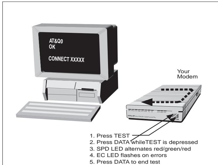
**Figure 10-1. Analog Loopback Self-Test**
